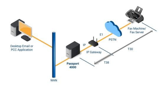
The organization in the diagram below has an Avaya VoIP solution in place linking its multiple international offices and has implemented FoIP with a virtualized Lane Passport Fax Server.
